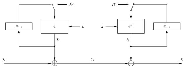
Fig. 5.5 Encryption and decryption in OFB mode
