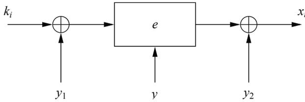
**Fig. 5.12** Key whitening of a block cipher
