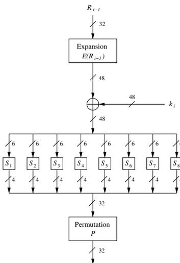
Fig. 3.10 Block diagram of the  $f$ -function
