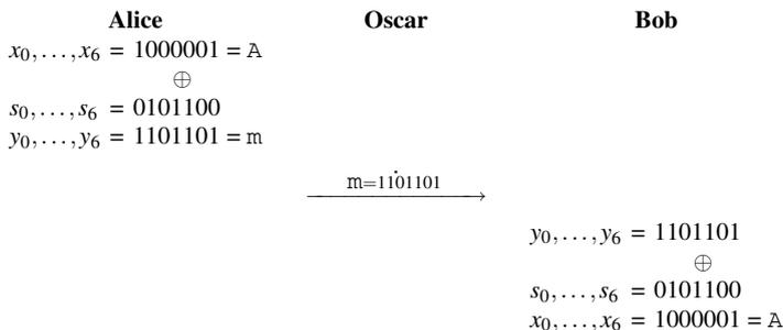
Note that the encryption by Alice turns the uppercase A into the lower case letter m. Oscar, the attacker who eavesdrops on the channel, only sees the ciphertext letter m. Decryption by Bob *with the same key stream* reproduces the plaintext A again.
