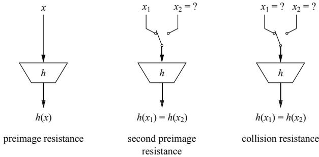
Fig. 11.4 The three security properties of hash functions
