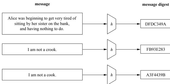
Fig. 11.3 Principal input–output behavior of hash functions
