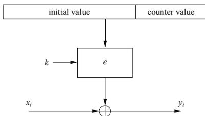
Fig. 5.7 Encryption and decryption in counter mode
