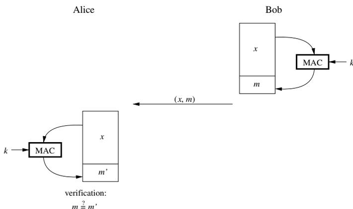
**Fig. 12.1** Principle of message authentication codes (MACs)
