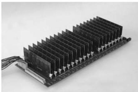
**Fig. 3.18** COPACOBANA — A cost-optimized parallel code breaker
