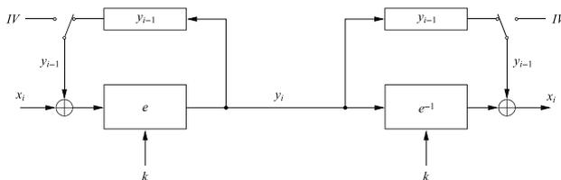
Fig. 5.4 Encryption and decryption in CBC mode
