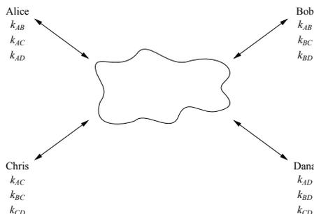
**Fig. 13.3** Keys in a network with  $n = 4$  users
