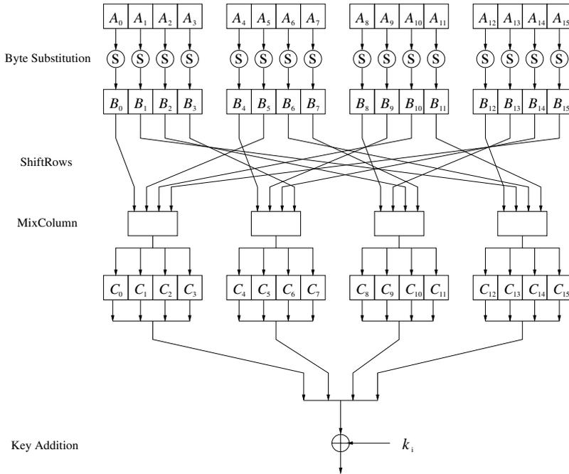
Fig. 4.3 AES round function for rounds  $1, 2, \dots, n_r - 1$
