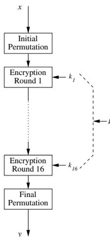
**Fig. 3.4** Iterative structure of DES
