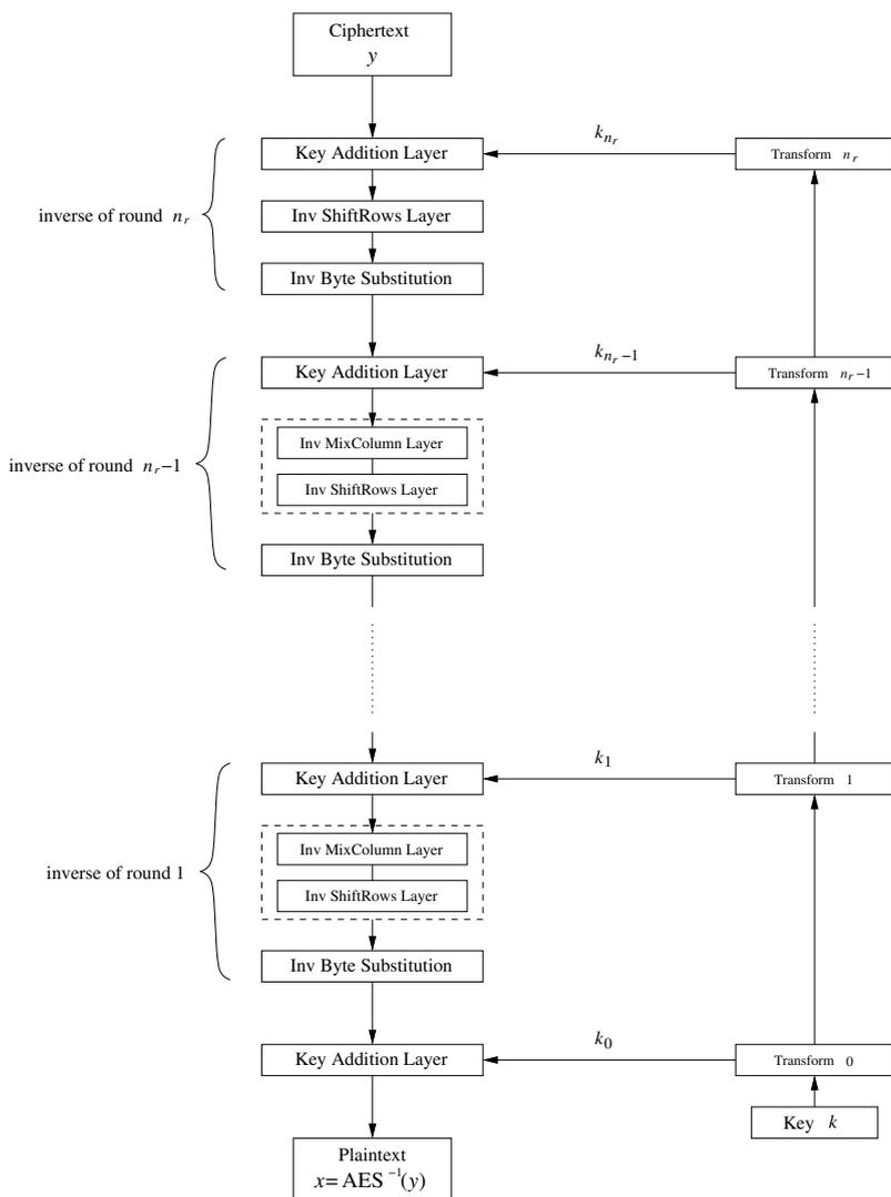
**Fig. 4.8** AES decryption block diagram
