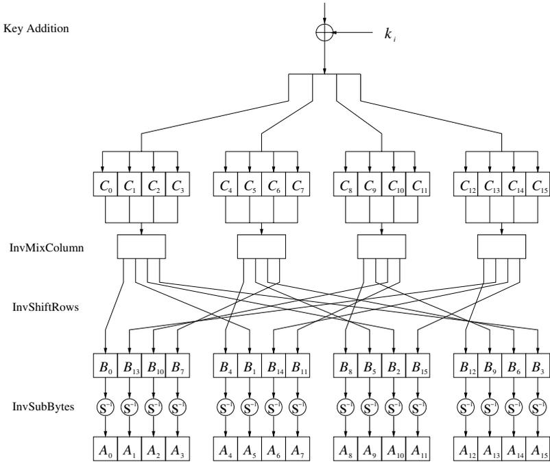
Fig. 4.9 AES decryption round function  $1, 2, \dots, n_r - 1$
