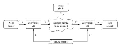
Fig. 1.5 Symmetric-key cryptosystem
