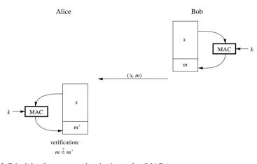
Fig. 12.1 Principle of message authentication codes (MACs)
