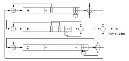
Fig. 2.8 Internal structure of the stream cipher Trivium
