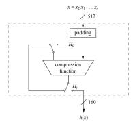
Fig. 11.9 High-level diagram of SHA-1
