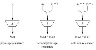
Fig. 11.4 The three security properties of hash functions
