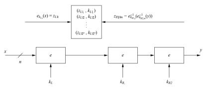
Fig. 5.11 Triple encryption and sketch of a meet-in-the-middle attack
