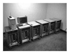
**Fig. 3.17** Deep Crack — the hardware exhaustive key-search machine that broke DES in 1998 (reproduced with permission from Paul Kocher)
