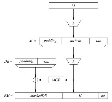
Fig. 10.2 Principle of EMSA-PSS encoding
