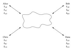
**Fig. 13.3** Keys in a network with n = 4 users
