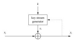
Fig. 2.3 Synchronous and asynchronous stream ciphers
