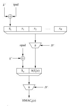
Fig. 12.2 HMAC construction
