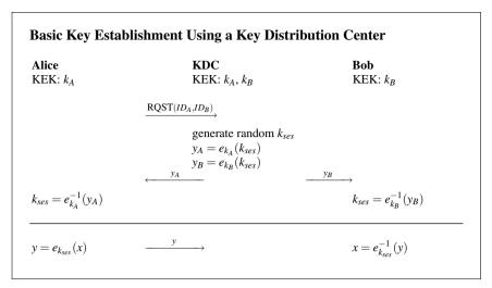
The protocol begins with a request message  $RQST(ID_A, ID_B)$ , where  $ID_A$  and  $ID_B$  simply indicate the users involved in the session. The actual key establishment protocol is executed subsequently in the upper part of the drawing. Below the solid line is, as an example, shown how Alice and Bob can now communicate with each other securely using the session key.
