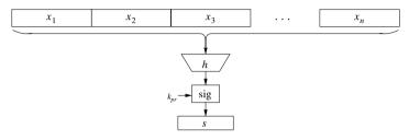
Fig. 11.2 Signing of long messages with a hash function
