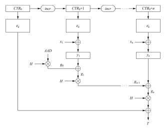
Fig. 5.8 Basic authenticated encryption in Galois Counter mode
