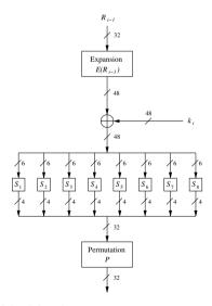
Fig. 3.10 Block diagram of the f-function
