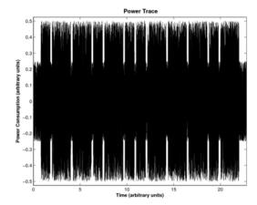
Fig. 7.5 Power consumption of an RSA decryption
