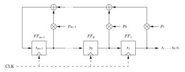
**Fig. 2.7** General LFSR with feedback coefficients  $p_i$  and initial values  $s_{m-1}, \ldots, s_0$
