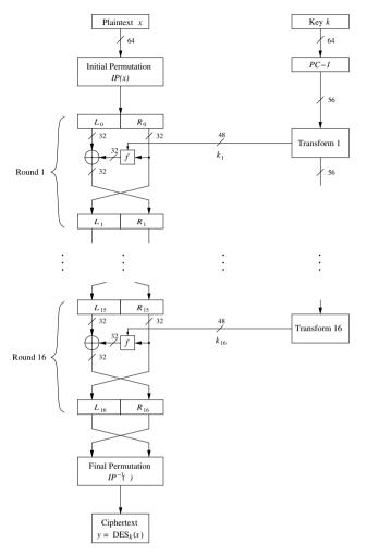
Fig. 3.5 The Feistel structure of DES
