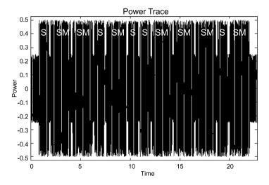
Fig. 7.4 The power trace of an RSA implementation
