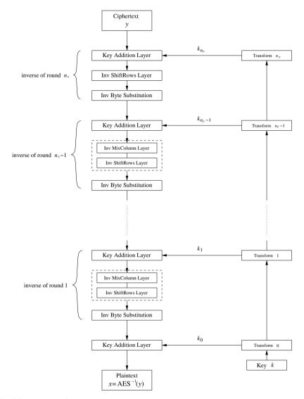
Fig. 4.8 AES decryption block diagram
