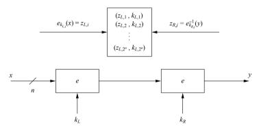
Fig. 5.10 Double encryption and meet-in-the-middle attack
