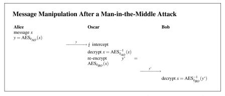
For illustrative purposes, we assumed that AES is used for the encryption. Of course, any other symmetric cipher can be used as well. Please note that Oscar can not only read the plaintext x but can also alter it prior to re-encrypting it with  $k_{BO}$ . This can have serious consequences, e.g., if the message x describes a financial transaction.
