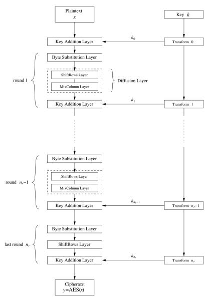
Fig. 4.2 AES encryption block diagram
